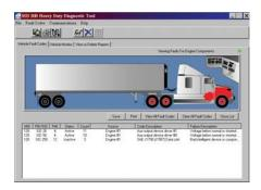
The MD-300 is the only diagnostic software on the market that includes a Graphic Vehicle Interface (GVI) that visually displays what components are reporting fault codes. Red indicates an active fault code, yellow indicates an inactive fault code, and green indicates no fault codes. You can instantly determine if a failure is affecting more than one system on the vehicle!
